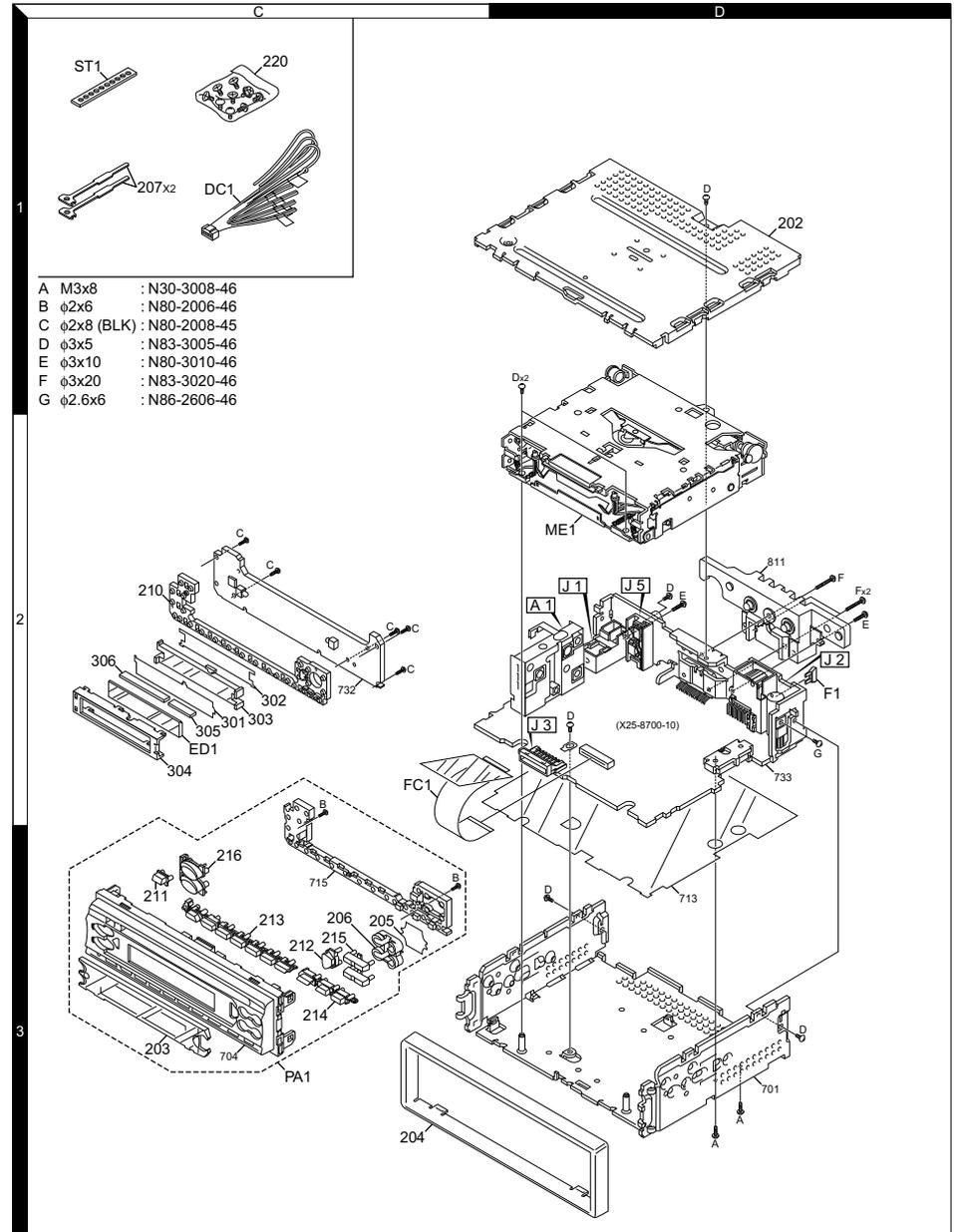
Parts with exploded numbers larger than 700 are not supplied.
